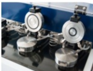
Measurement cell (Diameter 70mm, 30mm)
